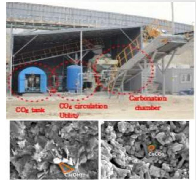
Figure 9.  $\text{Ca}(\text{OH})_2$  before carbonation
